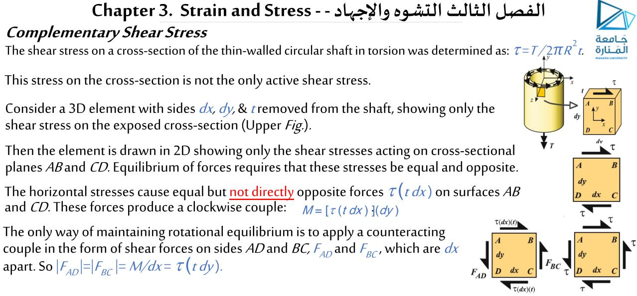
The shear stresses on *AD* & *BC* are equal and at right angles to the applied shear stress on *AB* & *CD*, so referred to as *complementary shear stresses*.
