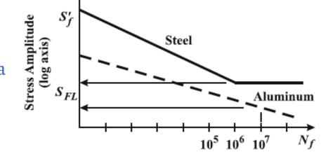
**Cycles to Failure (log axis)** Type equation here. For steels, the *fatigue limit*  $S_{FL}$  typically corresponds to a fatigue life of about  $10^6$  cycles. The S–N curve exhibits no further reduction and becomes horizontal.
