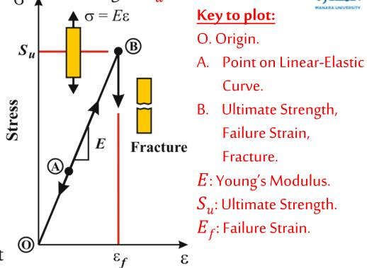
Gray cast iron exhibits some of the characteristics of ductile materials with a failure strain  $\varepsilon_f$  typically between [2Sy/E] and [5Sy/E]. Nevertheless, because the failure strain is small compared with ductile materials, gray cast iron is sometimes described as *semi-brittle*, sending a signal to the designer to proceed with caution.
