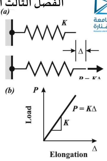
If the elongation (displacement) is too large, this linear relationship is no longer valid, which can be demonstrated by stretching a spring so much that it does not return to its original shape.
