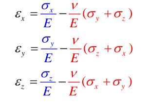
The normal strain in any direction is caused by the stress in that direction – the <u>direct stress</u> – and by the normal stresses in the two perpendicular directions due to the <u>Poisson effect</u>.
