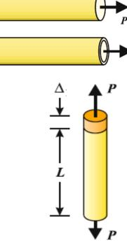
**Strain**: The *axial strain*  $\mathcal{E}$  – parallel to the axis – is the ratio of the bar's extension  $\Delta$  to its original length *L*. Hence,  $\mathcal{E} = \Delta/L$
