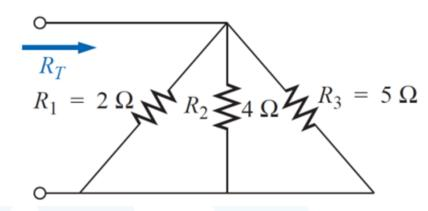
The total resistance of parallel resistors is always less than the value of the smallest resistor.
