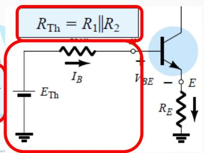
$$I_B = \frac{E_{\text{Th}} - V_{BE}}{R_{\text{Th}} + (\beta + 1)R_E}$$
