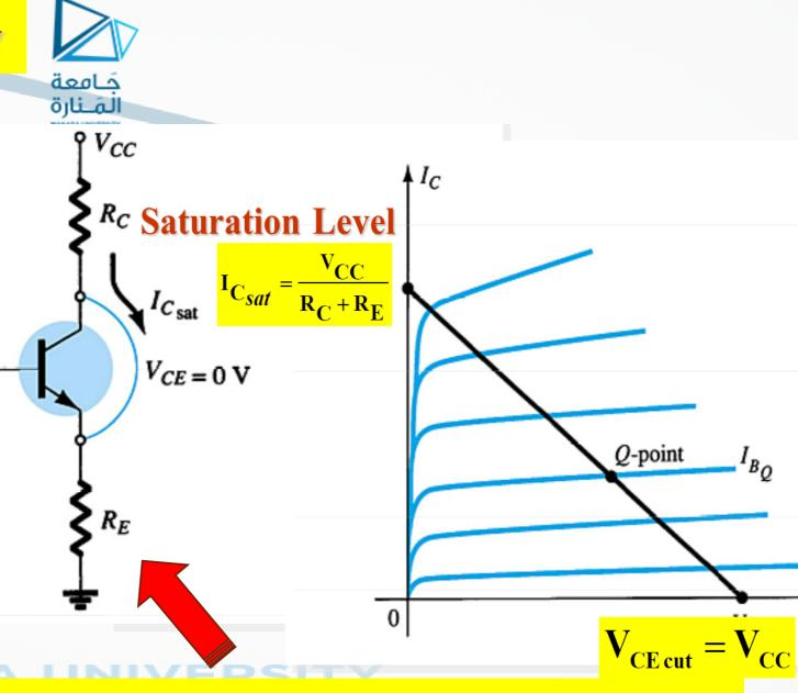
Adding Re to the emitter improves the stability of a transistor.
