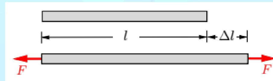
If the bar gets longer ( $\Delta l > 0$ ) the strain is positive; it is negative in the case of a shortening ( $\Delta l < 0$ )
