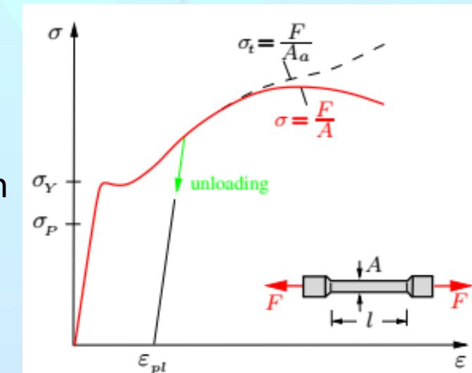
It is therefore appropriate to introduce the stress  $\sigma_t = F/Aa$  which is called *true stress* or *physical stress*. It represents the true stress in the region where necking takes place. The stress  $\sigma = F/A$  is referred to as *nominal* or *conventional* or *engineering stress*. The Fig. shows both stresses until fracture occurs.
