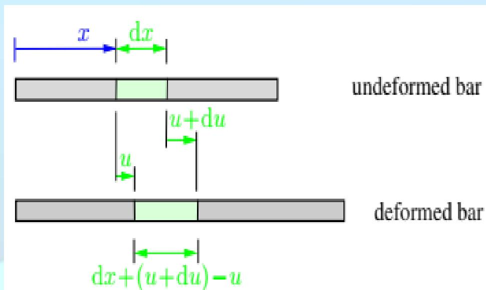
Instead of the whole we consider an element of the bar (Fig.). It has the length  $dx$  in the undeformed state. Its left end is located at  $x$ , the right end at  $x + dx$ .
