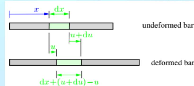
The displacement  $u(x)$  and the strain  $\varepsilon(x)$  describe the geometry of the deformation. Therefore they are called *kinematic quantities*. So the equation  $\varepsilon(x) = \frac{du}{dx}$  is referred to as a kinematic relation.
