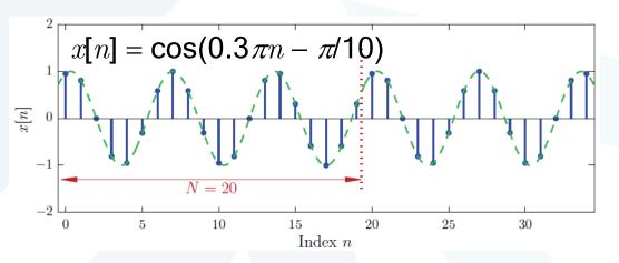
Example 5: Periodicity of a multi-tone discrete-time sinusoidal signal
