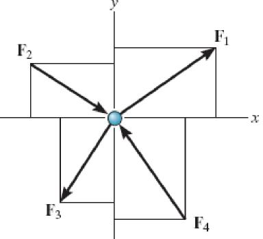
Scalar equations of equilibrium require that the algebraic sum of the x & y components to equal to zero.
