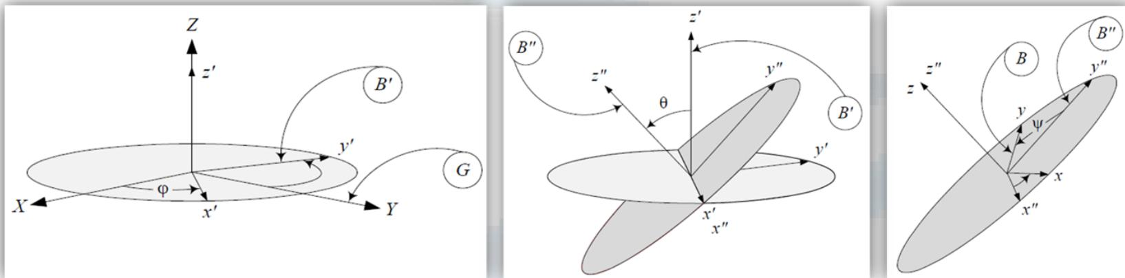
$$R = R_{z,\psi} \cdot R_{x_\psi,\theta} \cdot R_{z_\theta,\varphi}$$
