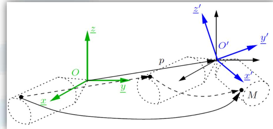
$$T = \begin{pmatrix} R & P \\ 0 & 1 \end{pmatrix} \Rightarrow T^{-1} = \begin{pmatrix} R^T & -R^T P \\ 0 & 1 \end{pmatrix}$$
