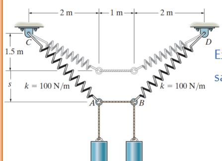
Ex. 2. Determine the mass of each of the two cylinders if they cause a sag of s = 0.5 m when suspended from the rings at A and B.
