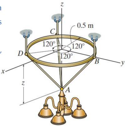
Example 4. The 50-kg pot is supported from A by the three cables.
