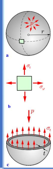
Now a thin-walled spherical vessel of radius r, subjected to a gage pressure p (Fig. a) is considered. Here, the stresses  $\sigma_t$  and  $\sigma_{\varphi}$  act in the wall (Fig. b). When the vessel is cut into half (Fig. c),  $\sigma_t$  is obtained from the equilibrium condition:
