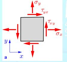
2. <u>Shear stresses</u> reach extreme values when  $d\tau_{\xi\eta}/d\varphi = 0 \Rightarrow -(\sigma_x - \sigma_y)\cos 2\varphi - 2\tau_{xy}\sin 2\varphi = 0$
