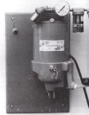
Fig. 12-10 Power-driven mechanical spatulator with a vacuum attachment. (From Craig RG, O'Brien WJ, Powers JM: Dental materials: properties and manipulation , ed 6, St Louis, 1996, Mosby.)
