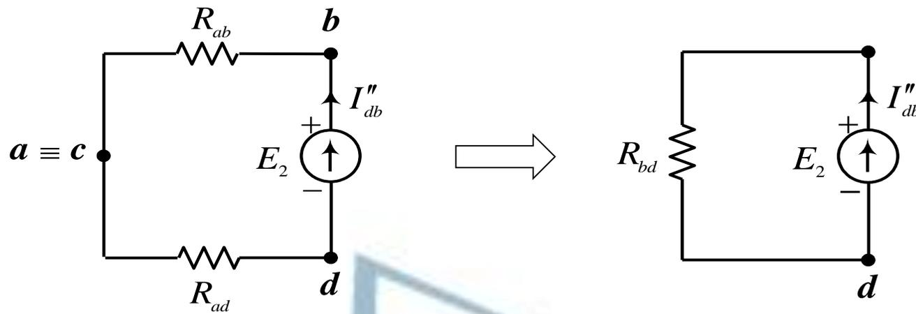
$$V''_{ab} = I''_{db} \cdot R_{ab} = 4 \times 10 = 40 [V]$$
