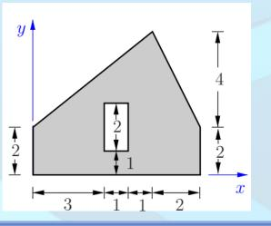
4. A wire with constant thickness is deformed into the depicted figure. The measurements are given in mm. Locate the centroid.
