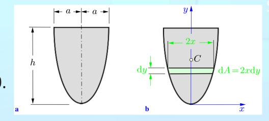
$$y_C = \frac{\int_A y dA}{A} = \frac{\int_A 2xy dy}{A}$$
