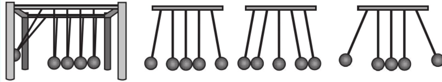
If one or more spheres is pulled away then released, it strikes the next sphere in the series and comes to (nearly) a complete stop. The impact force is transmitted through the group of spheres until an equal number of spheres on the opposite end is lifted by the reaction force. More than half the spheres can be set in motion. For example, three out of five spheres result in the central sphere swinging without any apparent interruption.
