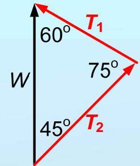
$$\frac{W}{\sin 75^\circ} = \frac{T_1}{\sin 45^\circ} = \frac{T_2}{\sin 60^\circ}$$
