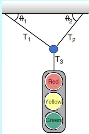
Example 1. If the traffic light weight is  $W=250\text{ N}$  and  $\theta_1=30^\circ$ ,  $\theta_2=45^\circ$ , find graphically the magnitudes  $T_1$  and  $T_2$ , representing the tensions in the two cables holding the traffic light. Then verify your answers using the sines formula.
