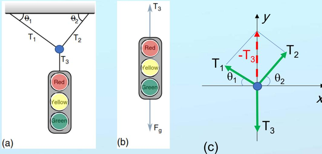
Free-body diagram of a traffic light suspension system;
