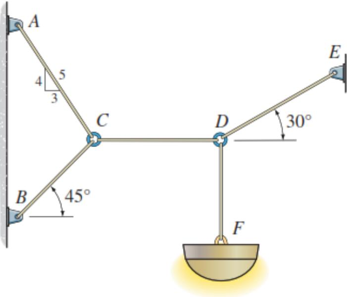
Ex.8. (1) Determine the tension developed in each cord required for equilibrium of the 20-kg lamp.
