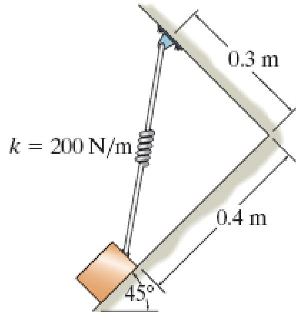
Ex.6. The block has a mass of 5 kg and rests on the smooth plane. Determine the unstretched length of the spring.
