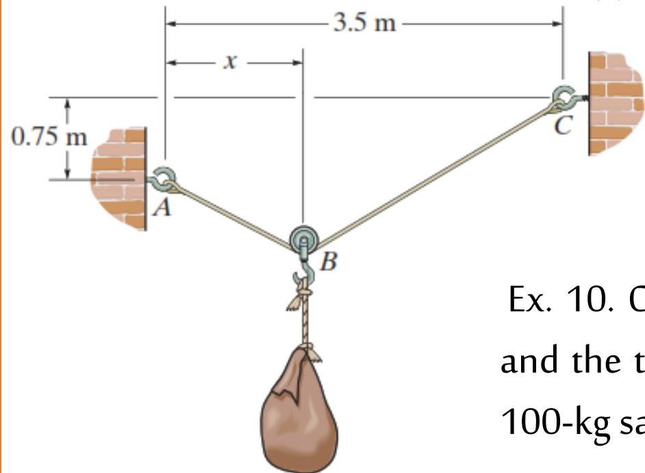
Ex. 10. Cable  $ABC$  has a length of  $5 \text{ m}$ . Determine the position  $x$  and the tension developed in  $ABC$  required for equilibrium of the  $100\text{-kg}$  sack. Neglect the size of the pulley at  $B$ .
