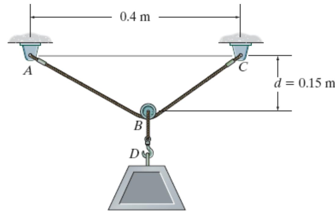
Ex.4. If cable CB is subjected to a tension that is twice that of cable CA, determine the angle for equilibrium of the 10-kg cylinder. Also, what are the tensions in wires CA and CB?
