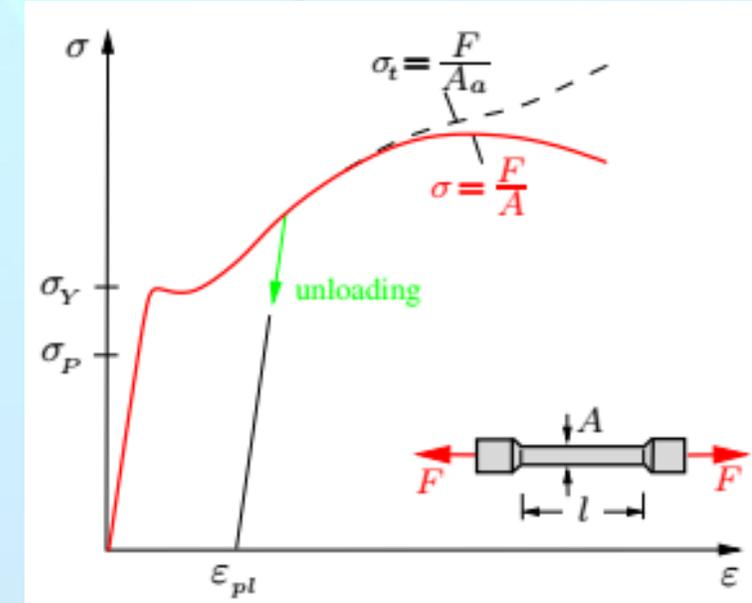
Experiments show that an elongation of the bar leads to a reduction of the cross-sectional area  $A$ . This phenomenon is referred to as *lateral contraction*.
