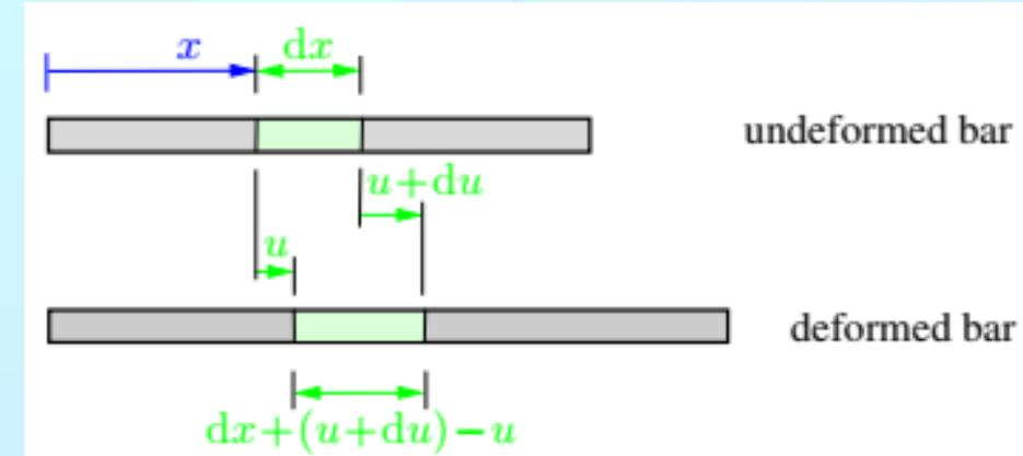
The displacement  $u(x)$  and the strain  $\epsilon(x)$  describe the geometry of the deformation. Therefore they are called *kinematic quantities*. So the equation  $\epsilon(x) = \frac{du}{dx}$  is referred to as a kinematic relation.
