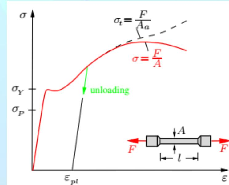
It is therefore appropriate to introduce the stress  $\sigma_t = F/A_a$  which is called *true stress* or *physical stress*. It represents the true stress in the region where necking takes place. The stress  $\sigma = F/A$  is referred to as *nominal* or *conventional* or *engineering stress*. The Fig. shows both stresses until fracture occurs.
