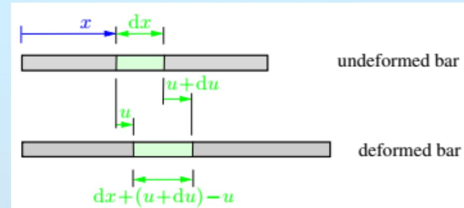
Instead of the whole we consider an element of the bar (Fig.). It has the length  $dx$  in the undeformed state. Its left end is located at  $x$ , the right end at  $x + dx$ .
