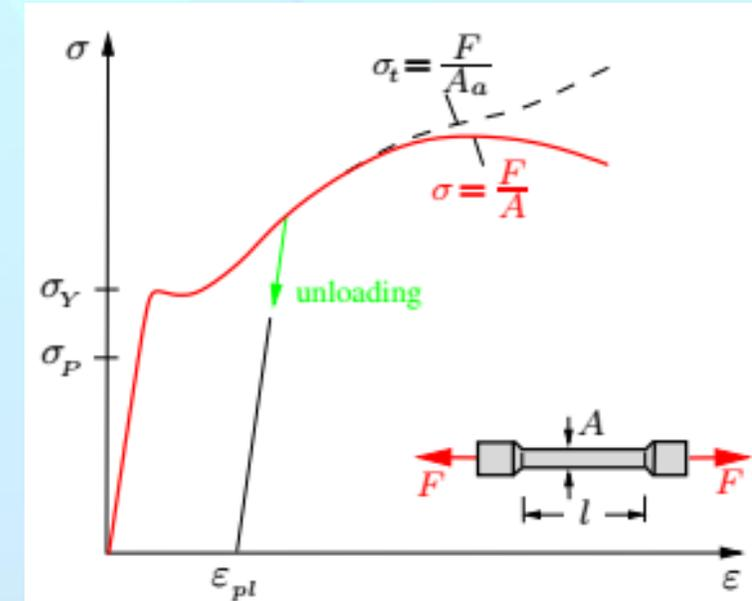
In the following we will always restrict ourselves to a linearly elastic material behavior. For the sake of simplicity we will refer to this behavior shortly as elastic, i.e., Then we have the linear relationship between the stress and the strain.
