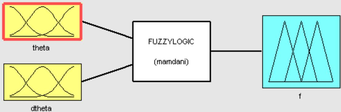
The diagram shows a fuzzy logic inference process. Two input membership functions, 'theta' and 'dtheta', are shown as yellow boxes with red borders. Each contains two overlapping bell-shaped curves. Lines connect these inputs to a central white box labeled 'FUZZYLOGIC (mandani)'. A line from this box connects to an output membership function 'f', shown as a cyan box with three overlapping triangular curves.
