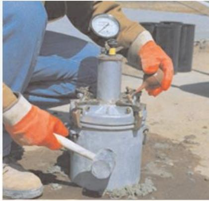
Pressure-type meter for determining air content.
