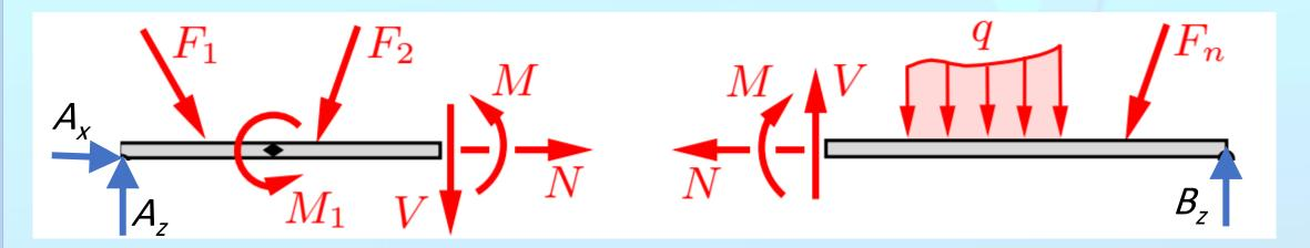
Since each part of the beam is in equilibrium, the 3 conditions of equilibrium for either part can be used to compute the three unknown stress resultants.
