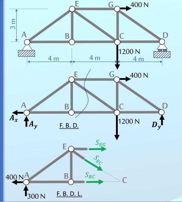
Determine the force in members EG, EC, and BC of the truss. Indicate whether the members are in tension or compression.
