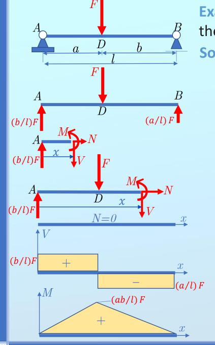
**Example 1.** Draw the diagrams of the stress resultants for the beam shown in figure.
