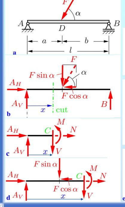
We will now determine the stress resultants for the simply supported beam shown in Fig.a.
