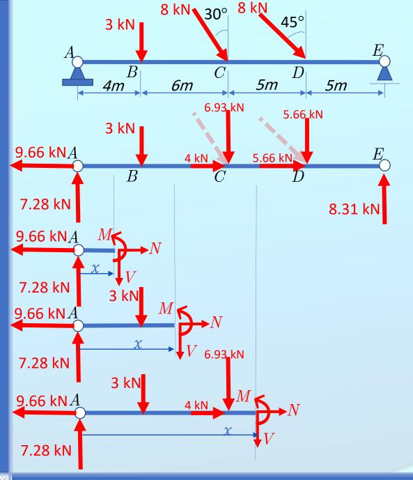
**Example 3.** Draw the diagrams of the stress resultants for the beam shown in figure.
