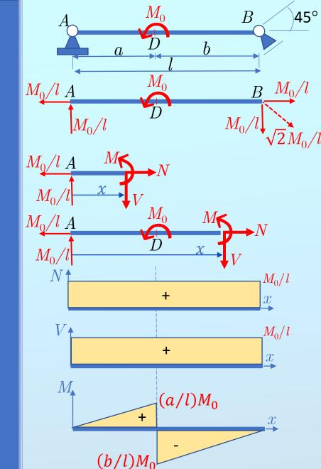
**Example 2.** Draw the diagrams of the stress resultants for the beam shown in figure.
