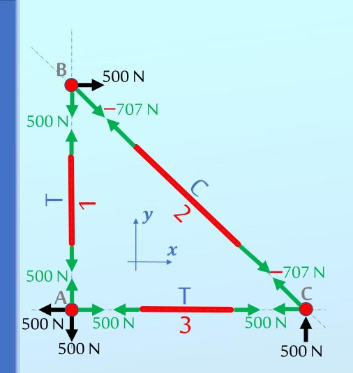
Determine the force in each member of the truss and indicate whether the members are in tension (T) or compression (C).
