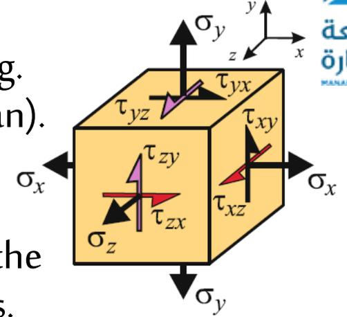
All of the stresses acting at a point are shown on the cube in Fig.; they are drawn in their positive senses as defined below.
