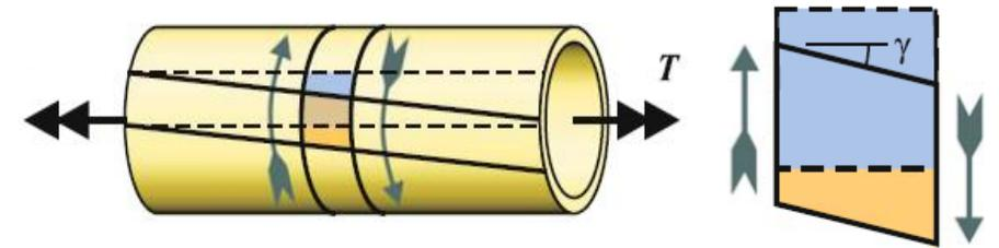
The torque deforms the dashed lines to the position of the solid angled lines. The square is transformed into a rhombus.
