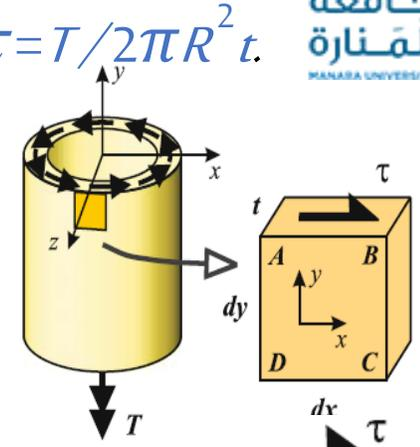
Then the element is drawn in 2D showing only the shear stresses acting on cross-sectional planes  $AB$  and  $CD$ . Equilibrium of forces requires that these stresses be equal and opposite.
