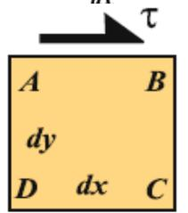
The only way of maintaining rotational equilibrium is to apply a counteracting couple in the form of shear forces on sides  $AD$  and  $BC$ ,  $F_{AD}$  and  $F_{BC}$ , which are  $dx$  apart. So  $|F_{AD}| = |F_{BC}| = M/dx = \tau(t dy)$ .
