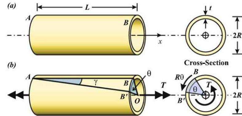
Experiments show that torque increases linearly with  $\theta$  for small (elastic) rotations. The shaft behaves as a *torsional spring*, with  $K_T$  as its *stiffness*. Then  $T = K_T \theta$ .
