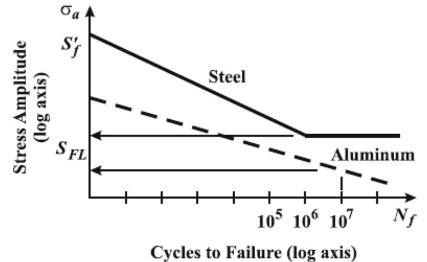
Type equation here. For steels, the ***fatigue limit***  $S_{FL}$  typically corresponds to a fatigue life of about  $10^6$  cycles. The S–N curve exhibits no further reduction and becomes horizontal.
