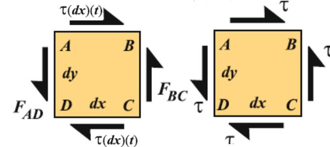
The shear stresses on  $AD$  &  $BC$  are equal and at right angles to the applied shear stress on  $AB$  &  $CD$ , so referred to as **complementary shear stresses**.
