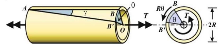
Now consider a square material element on the surface of the shaft initially bound by two dashed axial lines and two solid circumferential lines Fig.
