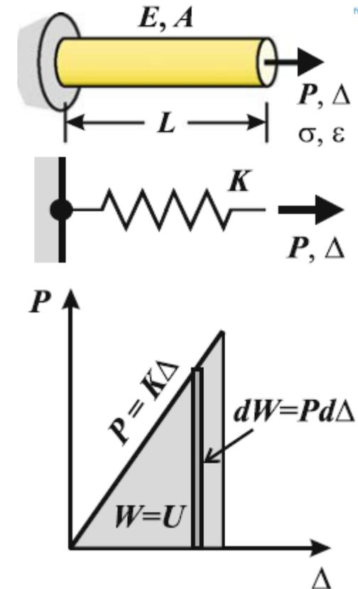
The maximum value of the *elastic strain energy density* is when the stress reaches the *yield strength*. The maximum elastic strain energy density is known as the *modulus of resilience*  $U_R$  : (معامل الممانعة الميكانيكية)
