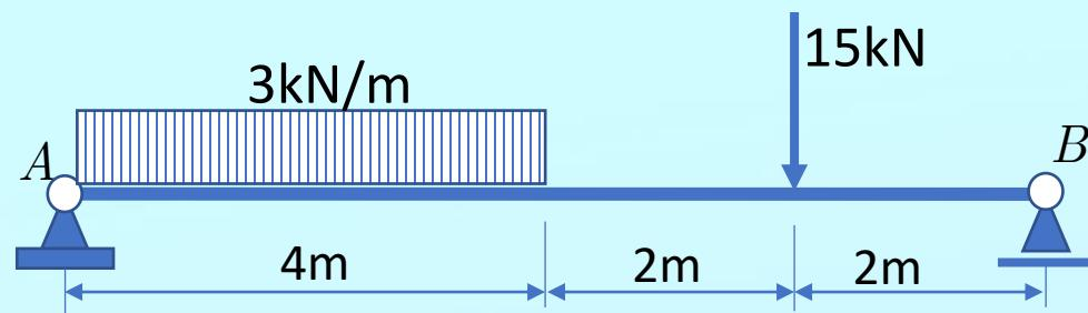
**Example 7** Determine the shear-force and bending-moment diagrams for the simple beam shown in Fig. using the section method.
