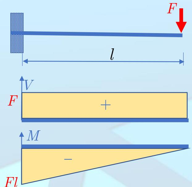
**Example 3** Determine the shear-force and bending-moment diagrams for the beam shown in Fig. using the section method and the integration method.
