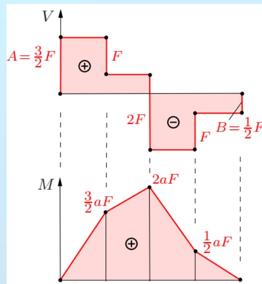
**Example 2** Determine the shear-force and bending-moment diagrams for the cantilever beam shown in Fig.a.
