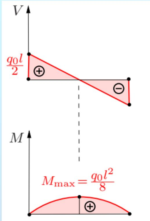
**Example 4** Determine the shear-force and bending-moment diagrams for the cantilever beam shown in Fig. using the section method and the integration method.
