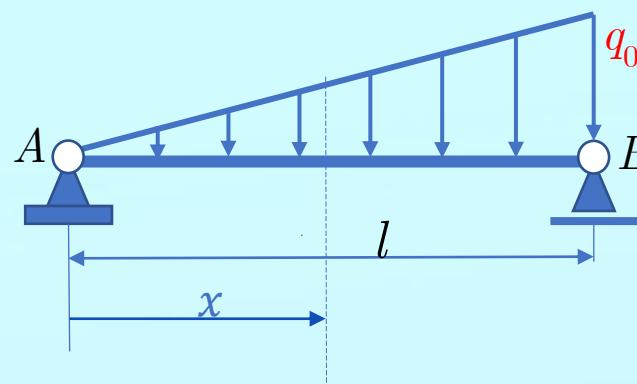
**Example 5** Determine the shear-force & bending-moment diagrams for the shown simple beam. using the integration method.
