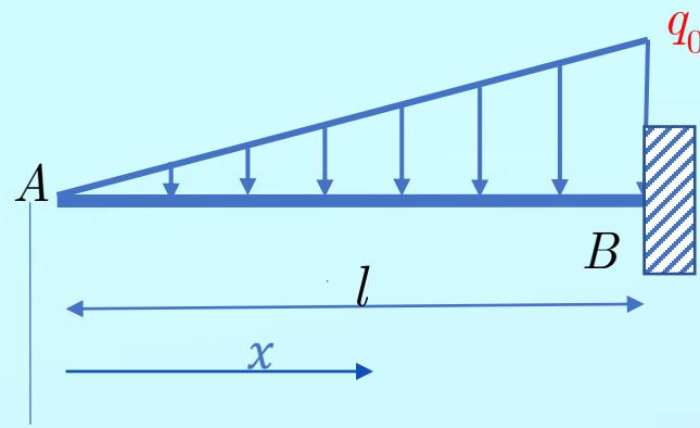
Example 6. Determine the shear-force & bending-moment diagrams for the shown cantilever beam, using the integration method.
