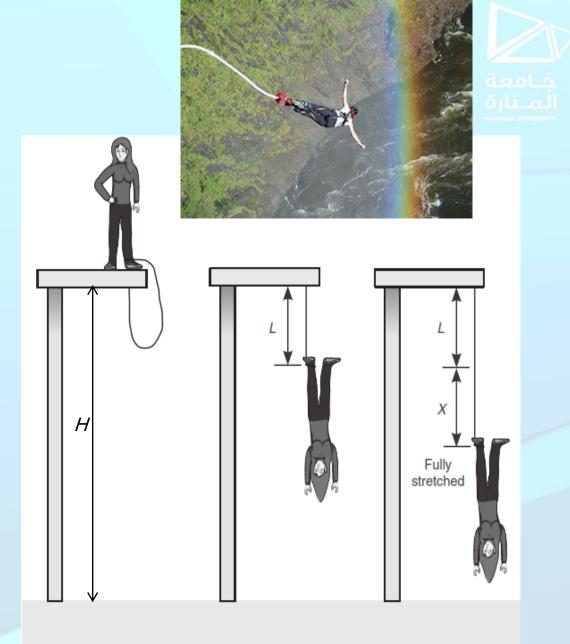
3. If the height of the tower is 60 m, and the weight of the person is 800 N, and the unstretched length L = 20 m, find a value of K that enables this person to stop exactly 2 m above the ground.
