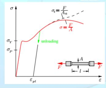
This continues until the stress reaches the *yield stress*  $\sigma_Y$ . From this point of the stress-strain diagram the strain increases at a practically constant stress: the material begins to *yield*. Note that many materials do not exhibit a pronounced yield point.
