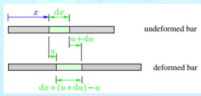
The displacement u(x) and the strain  $\varepsilon(x)$  describe the geometry of the deformation. Therefore they are called *kinematic quantities*. So the equation  $\varepsilon(x) = \frac{du}{dx}$  is referred to as a kinematic relation.
