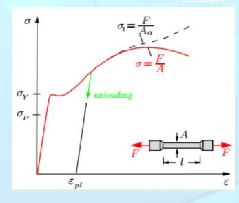
In the following we will always restrict ourselves to a linearly elastic material behavior. For the sake of simplicity we will refer to this behavior shortly as elastic, i.e., Then we have the linear relationship between the stress and the strain.
