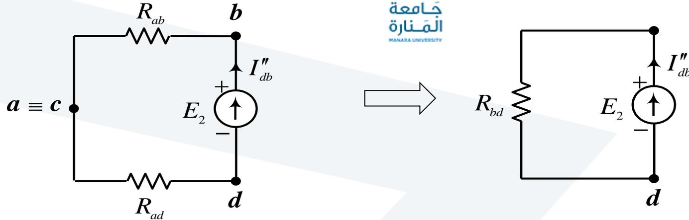
$$V_{ab}'' = I_{db}'' \cdot R_{ab} = 4 \times 10 = 40[V]$$
