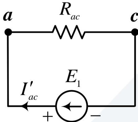
$$V'_{ab} = V'_{bc} = I'_{ac} \cdot R_{ab} = I'_{ac} \cdot R_{bc} = 5 \times 12 = 60[V]$$
