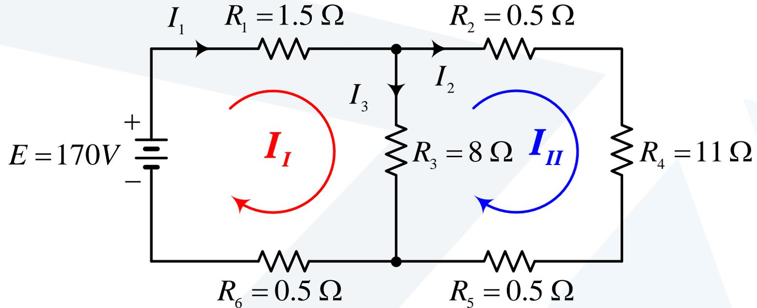
$$0 = I_{II} \cdot (R_2 + R_3 + R_4 + R_5) - I_I \cdot R_3$$
