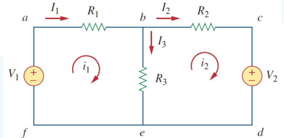
As the second step, we apply **KVL** to each mesh. Applying **KVL** to mesh 1, we obtain:
