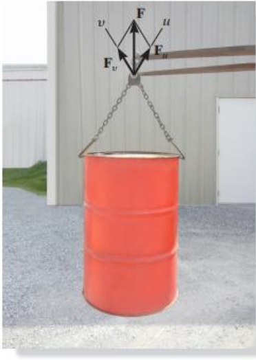
Using the parallelogram law the supporting force F can be resolved into components acting along the u and v axes.
