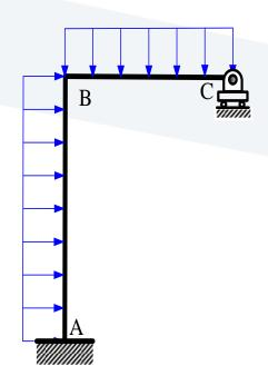
The frame is statically indeterminate to degree one. However, there are 3 kinematic unknowns,  $\theta_B$ ,  $\theta_C$  and  $\Delta$ , the horizontal displacement of B and C. Since we do not assume axial deformations to take place in the beams or columns: B and C must have the same horizontal displacement, and the vertical displacement at B is zero.
