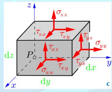
For example,  $\tau_{vx}$  is a shear stress acting in a section whose normal points in y-direction; the stress itself points in x-direction.
