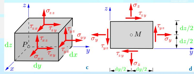
By means of the decomposition of the three stress vectors into their components we have obtained three normal stresses  $(\sigma_x, \sigma_y, \sigma_z)$  and six shear stresses  $(\tau_{xy}, \tau_{xz}, \tau_{yx}, \tau_{yz}, \tau_{zx}, \tau_{zy})$ . So nine stress components.
