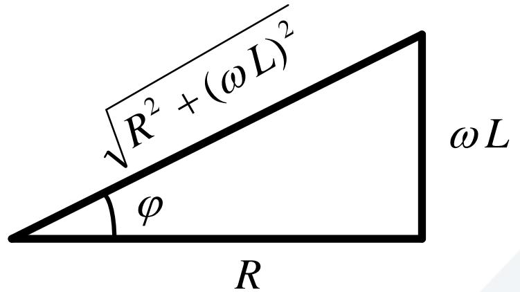
$$\tan \varphi = \frac{\sin \varphi}{\cos \varphi} = \frac{\omega L}{R} \Rightarrow \varphi = \arctan\left(\frac{\omega L}{R}\right)$$
