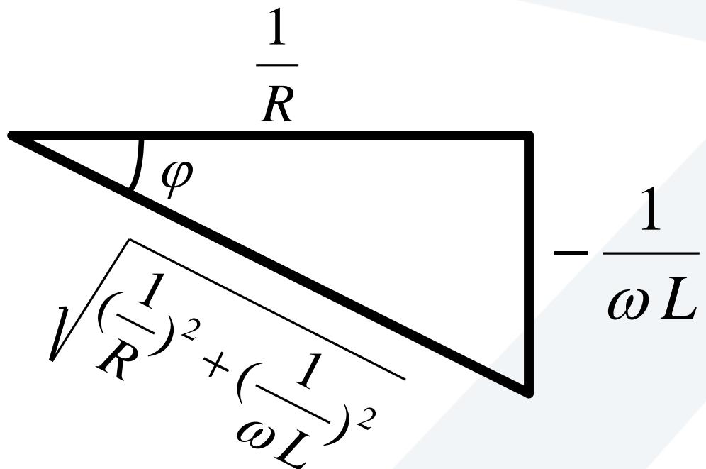
$$i = V_m \cdot \sqrt{\left(\frac{1}{R}\right)^2 + \left(\frac{1}{\omega L}\right)^2} \cdot \sin(\omega t - \operatorname{arctg}\left(\frac{R}{\omega L}\right))$$
