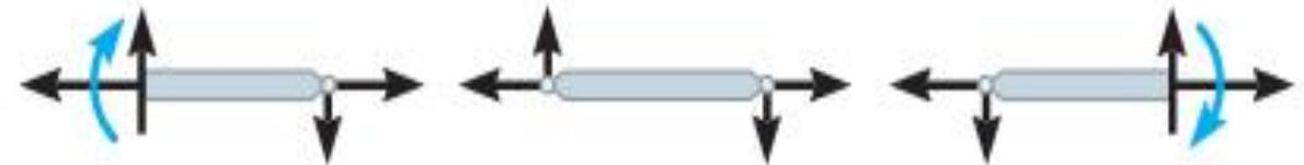
Statically indeterminate to the first degree
