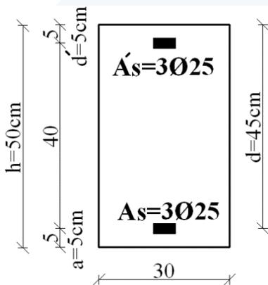
$$\left( \frac{N'_u}{\Omega} = 3000 \text{kN}, \frac{M_u}{\Omega} = 200 \text{kN.m} \right) -1$$
