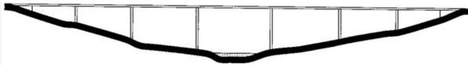
Continuous beam viaduct of uniform depth with varying spans
