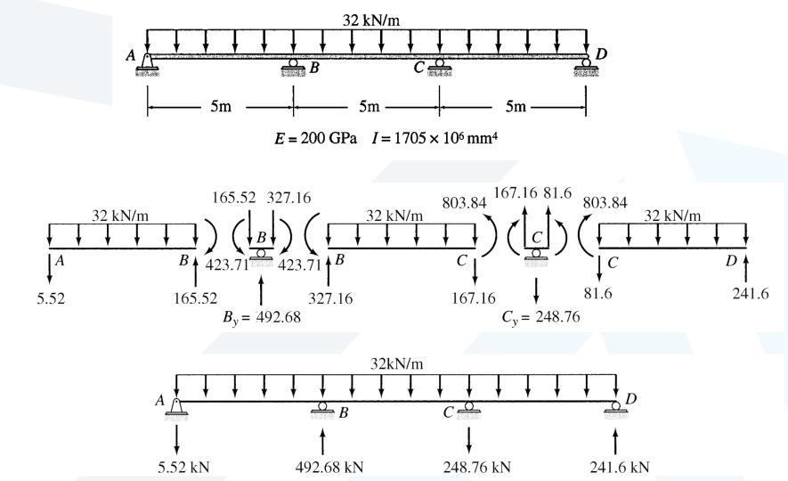
Ex.3: For the next frame under the given loads, by the slope-deflection method, calculate the reactions, and draw the bending moment, shear force & normal force diagrams. El is constant.
