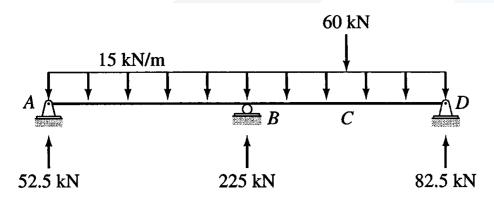
Ex.2: Determine the member end moments and reactions for the continuous beam shown in figure due to the uniformly distributed load and due to the support settlements of 15 mm at B, 36 mm at C, and 18 mm at D.
