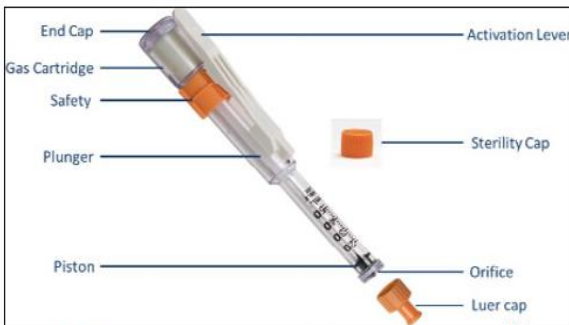
Figure 1. Components of a needle-less injection device [4]
