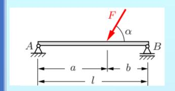
Solution: The beam is rigidly supported; the support A transmits two reactions and support B one reaction. In total, the three unknown reaction forces  $A_H$ ,  $A_V$  & B exist, therefore, the beam is statically determinate.
