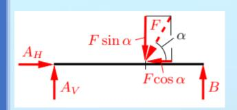
We free the beam from its supports and make the reaction forces visible in the free-body diagram where we choose their senses of direction along the action lines freely. Hence, the equilibrium conditions are given by
