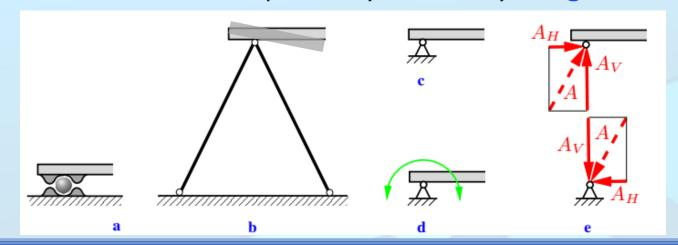
The rotational degree of freedom disappears if a support by two struts is complemented by an additional, somewhat shifted, third strut figure a.
