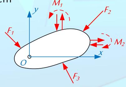
Since the number of unknowns must coincide with the number of equations, three unknown reactions (forces or couple moments) must exist at the supports: r = 3. It will be explained later that this necessary condition may not be sufficient for the determination of the support reactions.
