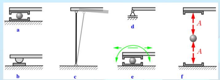
Supports that can transmit two reactions (r = 2). Examples of this type of support are
