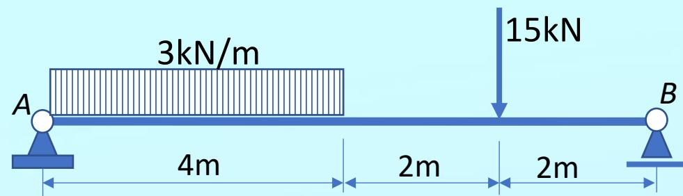
**Problem 5.** Determine the shear-force and bending-moment diagrams for the simple beam shown in Fig. using the section method.
