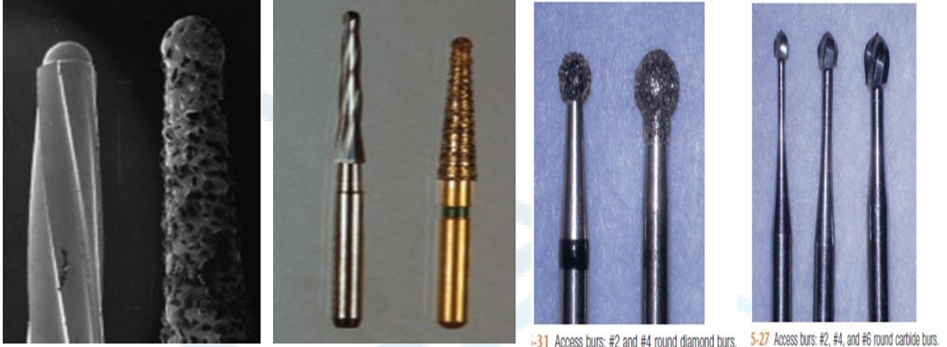
31 Access burs: #2 and #4 round diamond burs. 5-27 Access burs: #2, #4, and #6 round carbide burs.
