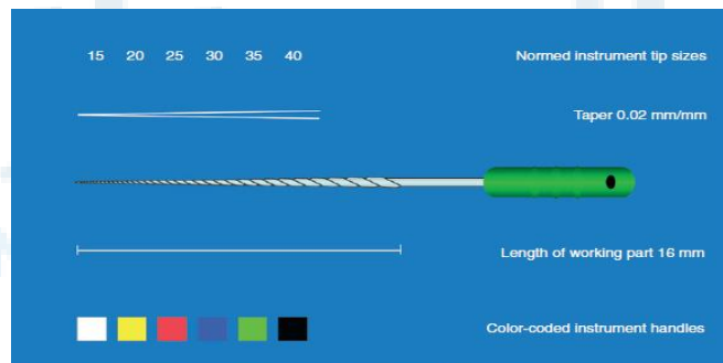
FIG. 6-15 Schematic drawing of an ISO-normed hand instrument size #35. Instrument tip sizing, taper, and handle colors are regulated by the ISO/ANSI/ADA norm.
