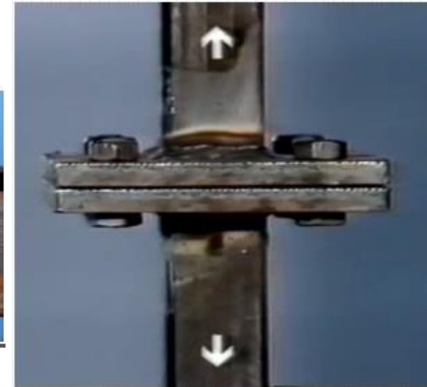
connections in tension ;
