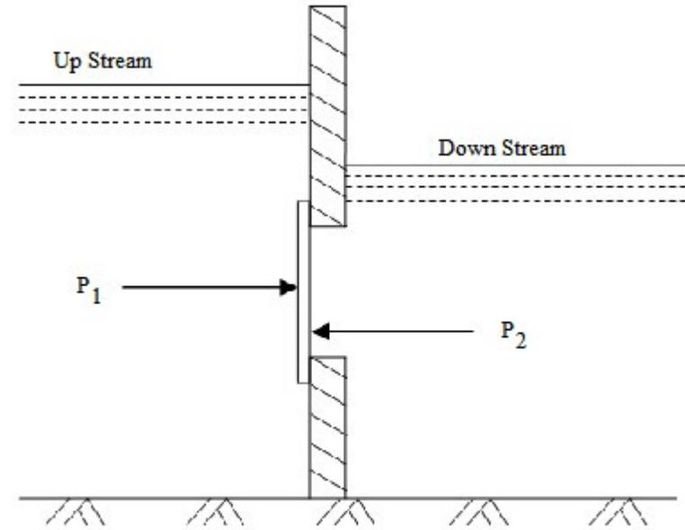
Fig : Sluice Gate
