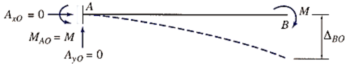
(b) Primary Beam Subjected to External Moment M
