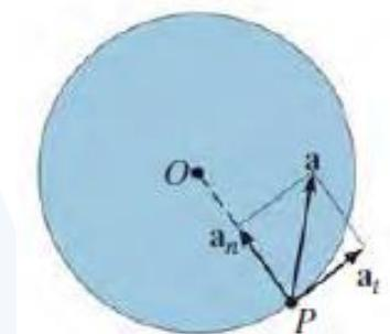
The *normal component of acceleration* represents the time rate of change in the velocity's direction. The *direction* of  $\mathbf{a}_n$  is always toward  $O$ , the center of the circular path
