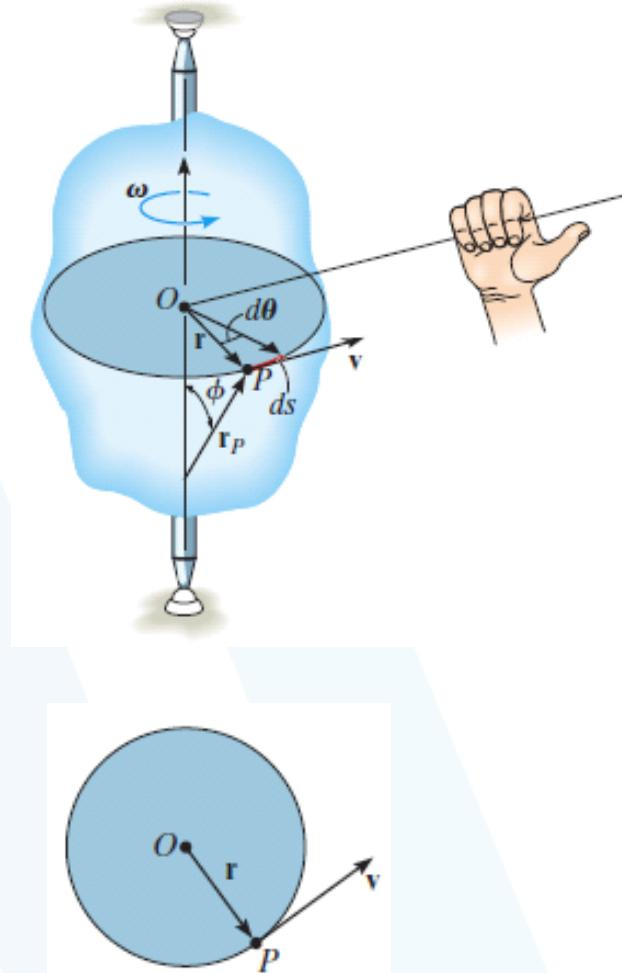
Both the magnitude and direction of  $\mathbf{v}$  can also be accounted for by using the cross product of  $\boldsymbol{\omega}$  and  $\mathbf{r}_P$ . Here,  $\mathbf{r}_P$  is directed from *any point* on the axis of rotation to point  $P$ . We have
