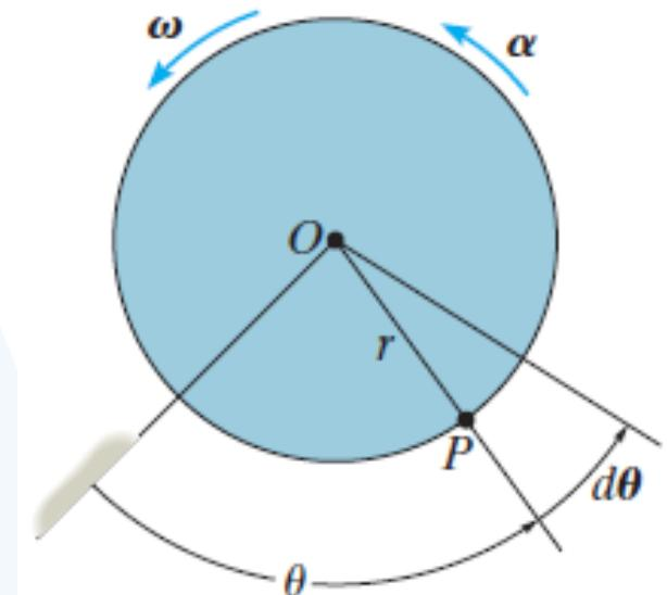
**Angular Velocity.** The time rate of change in the angular position is called the *angular velocity*  $\omega$  (omega). Since  $d\theta$  occurs during an instant of time  $dt$ , then,
