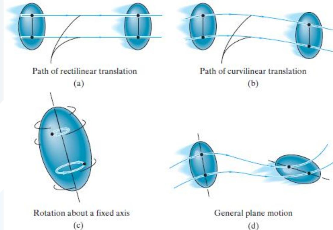
**Translation.** *This type of motion occurs when a line in the body remains parallel to its original orientation throughout the motion. When the paths of motion for any two points on the body are parallel lines, the motion is called *rectilinear translation*. If the paths of motion are along curved lines, the motion is called *curvilinear translation*.*
