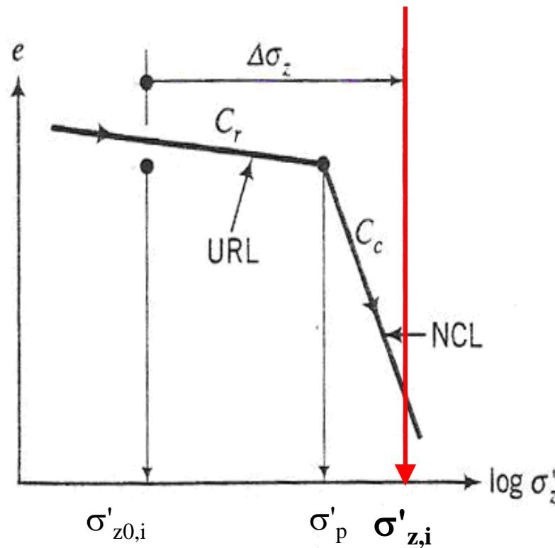
$$S_i = \frac{h_i}{1+e_0} \left( C_r \log \frac{\sigma'_p}{\sigma'_{z0,i}} + C_c \log \frac{\sigma'_{z0,i} + \Delta\sigma_{z,i}}{\sigma'_p} \right)$$
