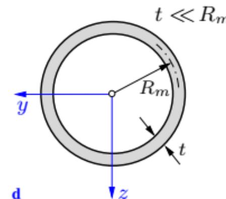
**Example 1** The cross section of a cantilever beam ( $l = 3 \text{ m}$ ) consists of a circular ring ( $R_i = 4 \text{ cm}$ ,  $R_a = 5 \text{ cm}$ ) The allowable stress is given by  $\sigma_{allow} = 150 \text{ MPa}$ . Determine the allowable value of the load  $F$ .
