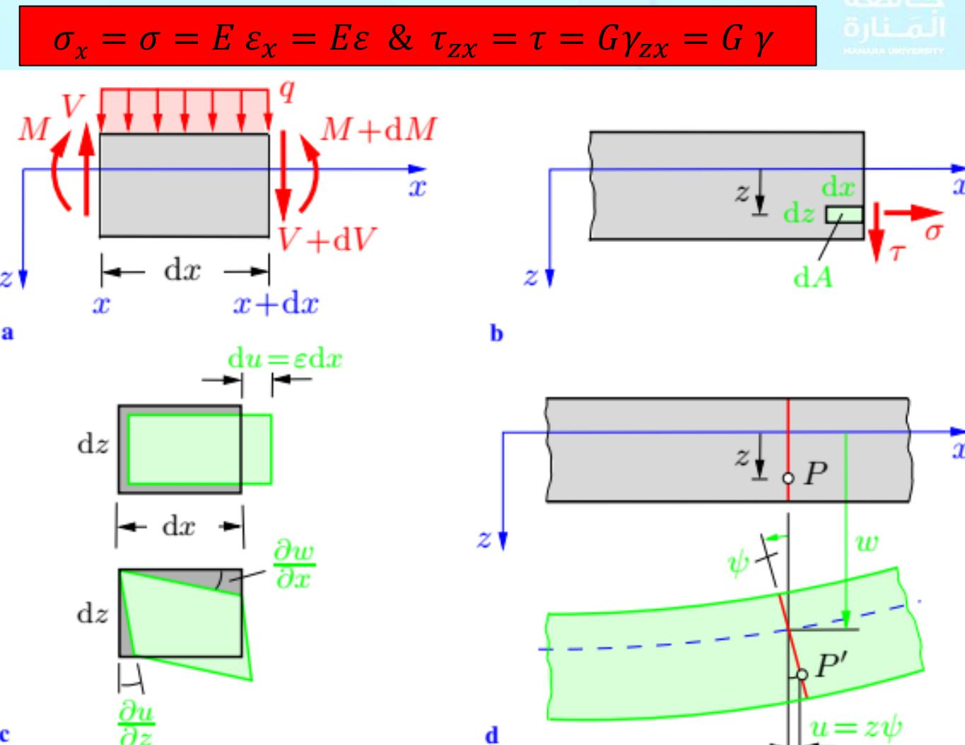
The displacement  $u$  of a point  $P$  which is located at a distance  $Z$  from the  $x$ -axis is given by  $u(x, z) = \psi(x) z$ .
