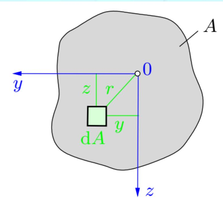
Frequently, an area  $A$  is composed of several parts  $A_i$  the moments of inertia of which are known (Fig.). In this case, the moment of inertia about the  $y$ -axis, for example, is obtained as the sum of the moments of inertia  $I_{y_i}$  of the individual parts about the *same axis*.
