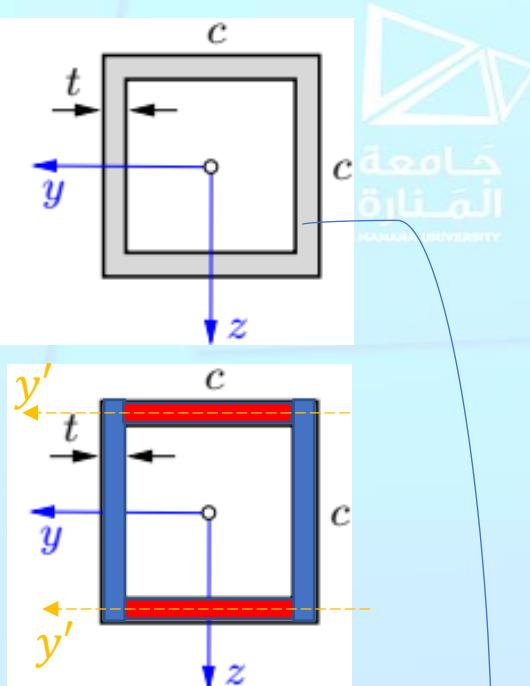
**Example 3** The simply supported beam (length  $l = 9 \text{ m}$ ) carries the force  $F = 210 \text{ kN}$ . Find the required side length  $C$  of the thin-walled quadratic cross section such that the allowable stress  $\sigma_{allo} = 200 \text{ MPa}$  is not exceeded. The thickness  $t = 12 \text{ mm}$  of the profile is given
