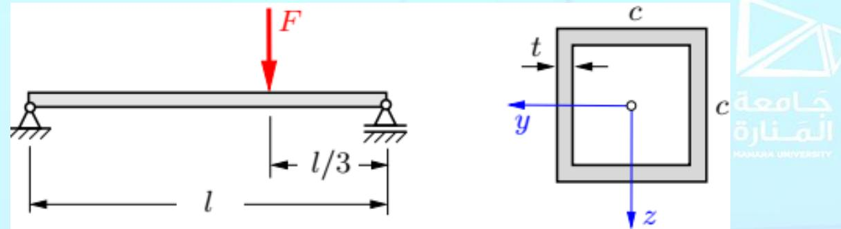
**Example 2** The simply supported beam (length  $l = 10 \text{ m}$ ) carries the force  $F = 200 \text{ kN}$ . Find the required side length  $C$  of the thin-walled quadratic cross section such that the allowable stress  $\sigma_{allo} = 200 \text{ MPa}$  is not exceeded. The thickness  $t = 15 \text{ mm}$  of the profile is given
