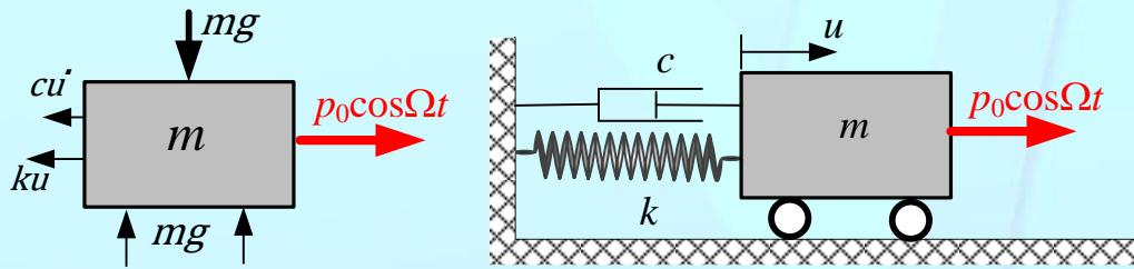
$$m\ddot{u} + cu + ku = p_0 \cos \Omega t \quad \ddot{u} + 2\xi\omega_n \dot{u} + \omega_n^2 u = (p_0 / m) \cos \Omega t$$
