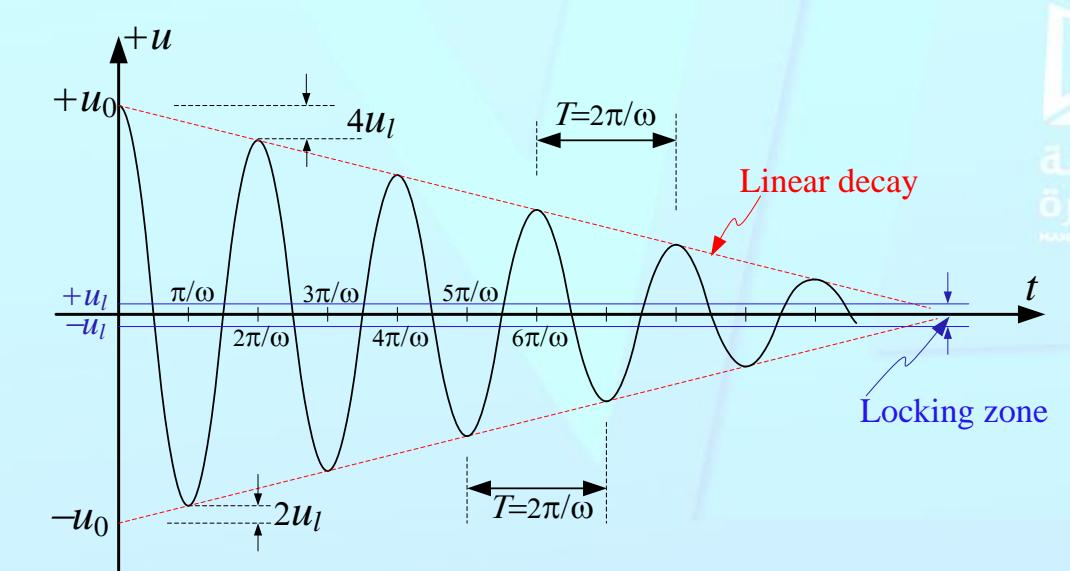
Ex. 3. For the system shown in figure,  $m = 500 \text{ kg}$ ,  $k = 400 \text{ kN/m}$ ,  $\mu = 0.15$  and the initial conditions are:  $u_0 = 16 \text{ cm}$ ,  $\dot{u}_0 = 0$ . Determine the amplitude after 8 half-cycles and the number of half-cycles of motion completed before the mass comes to rest
