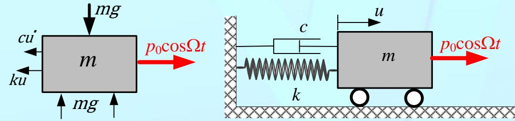
Example 1:  $\omega_n = 2\pi$  [rad/sec],  $\Omega = 0.4\pi$  [rad/sec],  $\xi = 5\%$ ,  $u_{st} = 25\text{mm}$ ,  $u_0 = 0$ ,  $\dot{u}_0 = u_{st} \omega_n$
