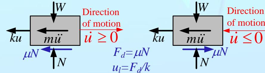
Any initial displacement greater than the locking one,  $u_l = F_d / k$ , can put the system in free vibration regime.
