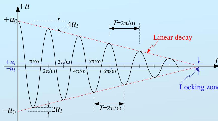
$$u(t) = A \cos(\omega t) + B \sin(\omega t) - (\text{sign}(\dot{u})) u_l$$
