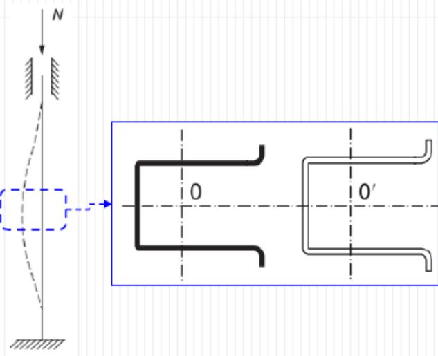
Cruciform sections, T-sections, angles and, in general, all cross-sectional shapes in which all the elements converge into a single point, are generally sensitive to torsional buckling phenomena.
