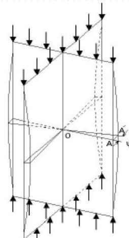
Cross-sections with one axis of symmetry are prone to flexural-torsional buckling in many cases instead of the torsional one, owing to the fact that both cross-sectional centroid and shear center lie on the axis of symmetry but are often not coincident.
