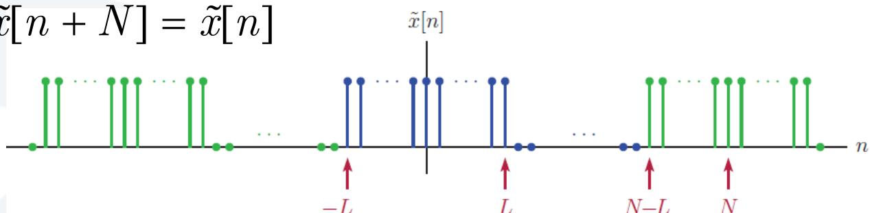
$$\tilde{c}_k = \frac{1}{N} \sum_{n=-L}^L e^{-j(2\pi/N)kn} = \frac{1}{N} \frac{e^{j(2\pi/N)Lk} - e^{-j(2\pi/N)(L+1)k}}{1 - e^{-j(2\pi/N)k}} \times \frac{e^{-j\pi k/N}}{e^{-j\pi k/N}}$$
