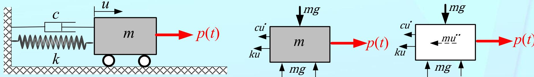
An harmonic excitation can be described either by means of a sine function:  $p(t) = p_0 \sin \Omega t$ , or by means of a cosine function:  $p(t) = p_0 \cos \Omega t$ .
