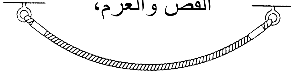
Cables support their loads in tension
